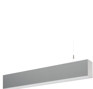
3 Maße (LxBxH): ca. 1500mm*70mm*120mm 4000K, 6150lm, Pendelleuchte UK = 2550 mm OKFFB
