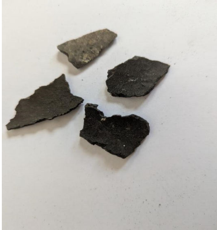
Foto 23: Schurf 6 Materialprobe (Asbest)
